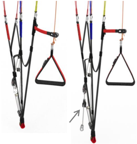
Fig. 3 MIURA 2 RS riser without speed limiter
