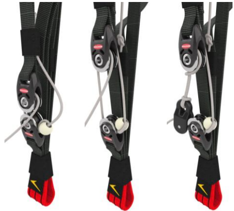
Fig. 8 MIURA 2 RS riser at speed steps with and without speed limiter
